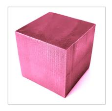
Examination of deflection in accordance to DIN EN 826, between two stiff panels. Illustration based on the third loading, Velocity of loading and unloading 20 seconds. Tested at room temperature. Dimensions of test specimens 50 mm x 50 mm x 50 mm x 50 mm.
