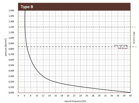
Natural frequency of a single-degree-of-freedom system (SDOF system) considering the dynamic stiffness of **Type B** on a rigid base. Dimensions of test specimens 50 mm x 50 mm.
