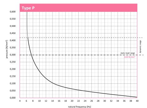
Natural frequency of a single-degree-of-freedom system (SDOF system) considering the dynamic stiffness of Type P on a rigid base. Dimensions of test specimens  $50 \, \text{mm} \times 50 \, \text{mm} \times 50 \, \text{mm}$ .
