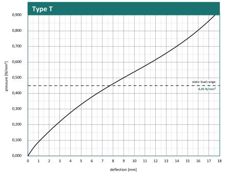
Examination of deflection in accordance to DIN EN 826, between two stiff panels. Illustration based on the third loading.
