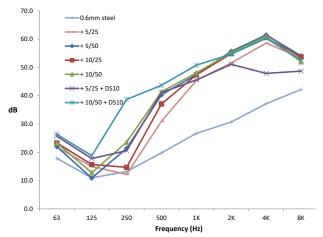
Acoustic duct lagging is a complex subject with the size, shape, thickness and configuration of the ductwork all having a significant effect on the system performance. The data shown above is based on flat panel tests used for SUPERLAG® Prime Flexilag products.
