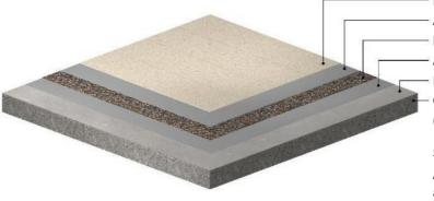
LVT or Vinyl sheeting Approved REGUPOL adhesive<sup>2</sup> **REGUPOL sonus multi 530** Approved REGUPOL adhesive<sup>2</sup> REGUPOL barrier 99-201<sup>3</sup> Concrete slab (prepared for floor finishes)
